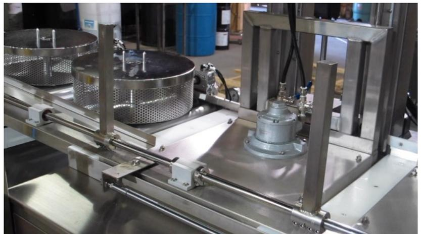
The first basket of parts is indexed to the Ultrasonic Cleaning Tank with the included Multiple Basket Transfer Automation System, which transfers multiple baskets in under 20-30 seconds, another benefit of the VORTEX design. Slow tumbling systems move only 1 basket at a time, which drastically extends the required cleaning time per basket. The MBT system included on the VORTEX moves all baskets simultaneously for faster throughput.
