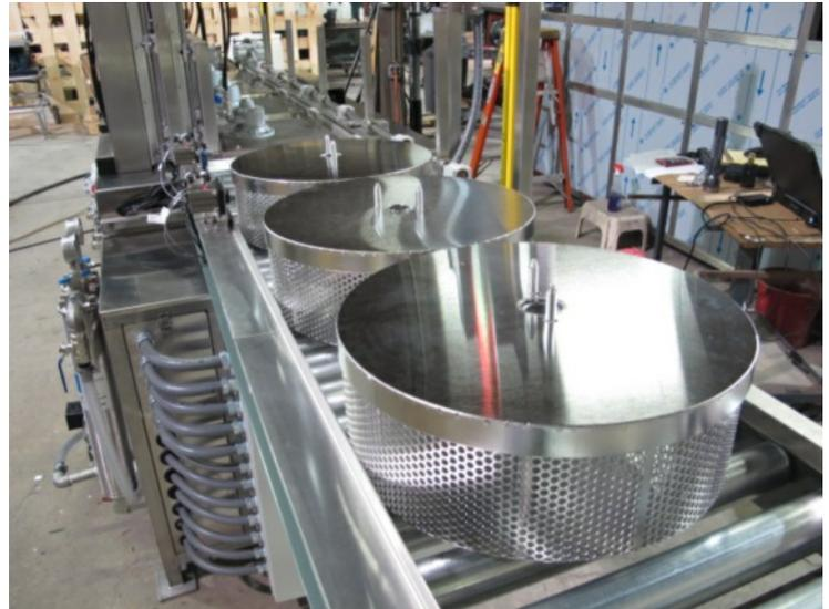
During the rotation, parts shuffle gently to the edge of the basket, and are held in place by centrifugal force. There is no damaging parts as that which occurs with tumbling as used in competitive designs. Even the most sensitive components can be safely cleaned in the VORTEX.
