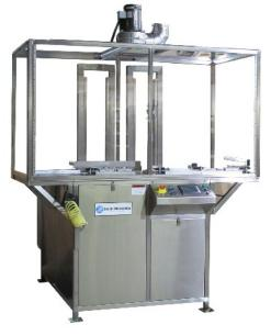
multi-position conveyor which allows queuing of multiple baskets and programmable recipe control.
